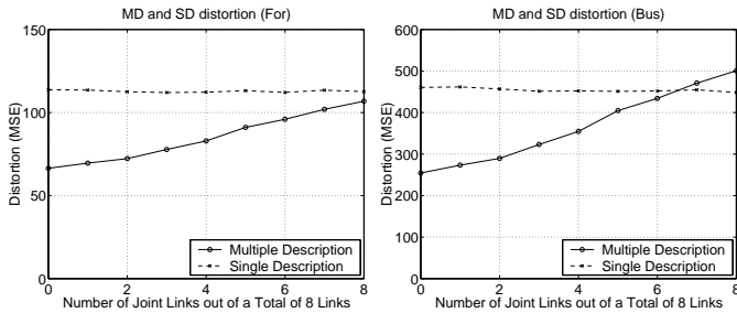
Fig. 5. MD versus SD distortion for a symmetric “Y”, as we vary the number of joint links given that the total number of links is 8. MD provides less distortion than SD for all cases of Foreman (right) and almost all cases for Bus (left) except where the paths are almost completely joint.
